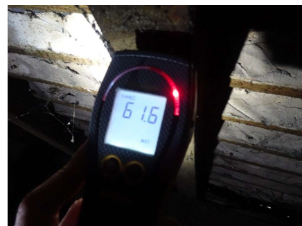
View of moisture meter reading indicating a saturated 'wet' condition.
